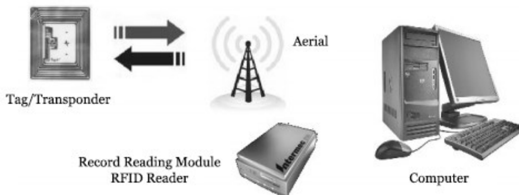
Figure 2. Elements of RFID system. Adapted from: Milanowicz, 2012.
