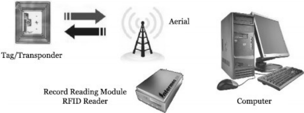
Figure 2. Elements of RFID system. Adapted from: Milanowicz, 2012.
