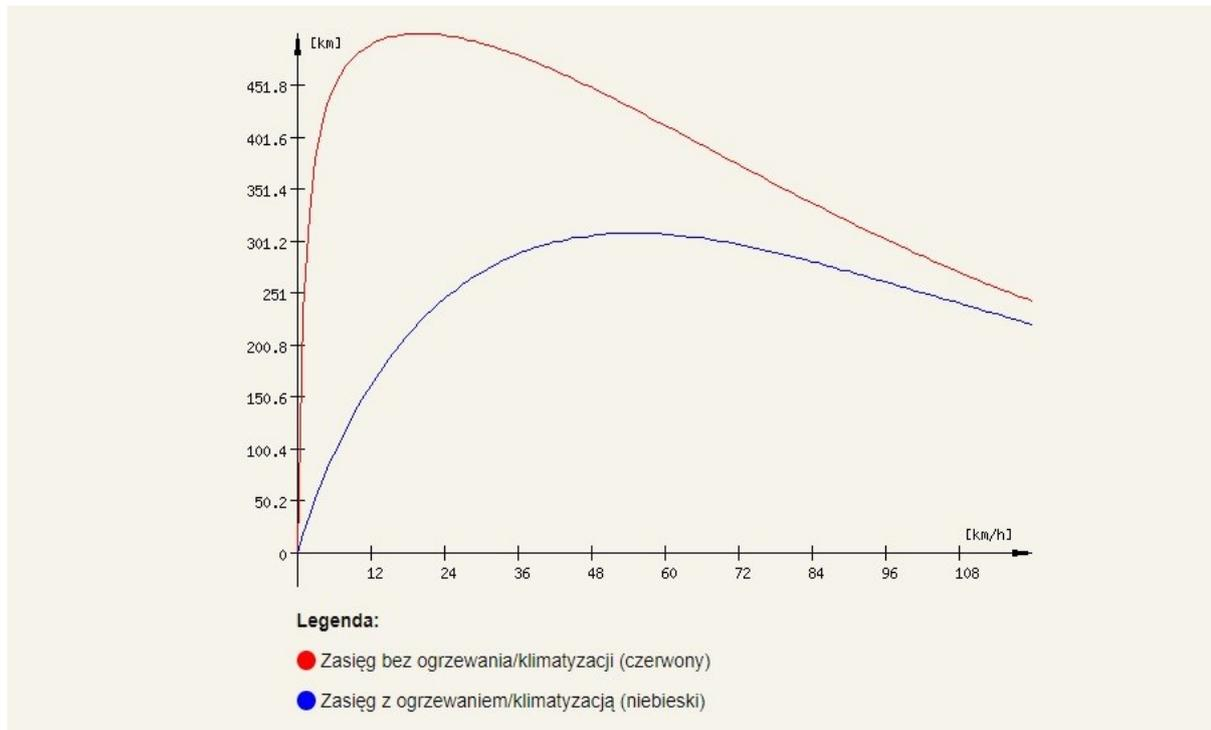
**Figure 2.** Example characteristics of the range of an electric vehicle in speed function source. Source: <https://samochodyelektryczne.org>.
